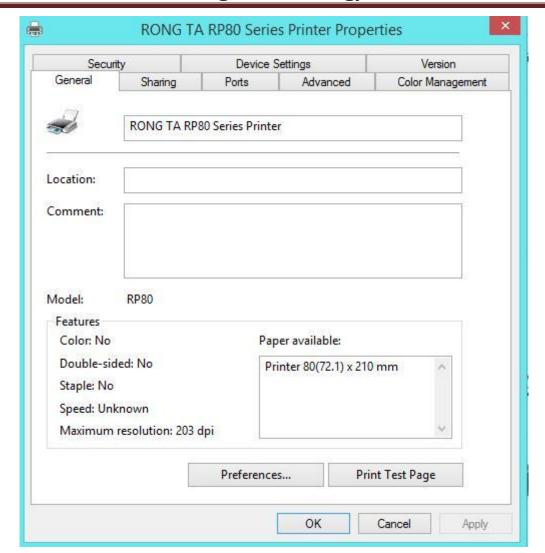
On RONG TA 80mm Series Printer Properties "General", you could configure the printer communication port, such as Serial port, Parallel port and USB port. You also could set the paper specification, beeper etc.
